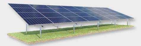
Efficiency even in small spaces! Not least because of the increased number of modules per table, the **Type 17R** system is very popular. The robust construction offers a space-saving, stable and safe rack system. The module tilt angle is 20°-25°
